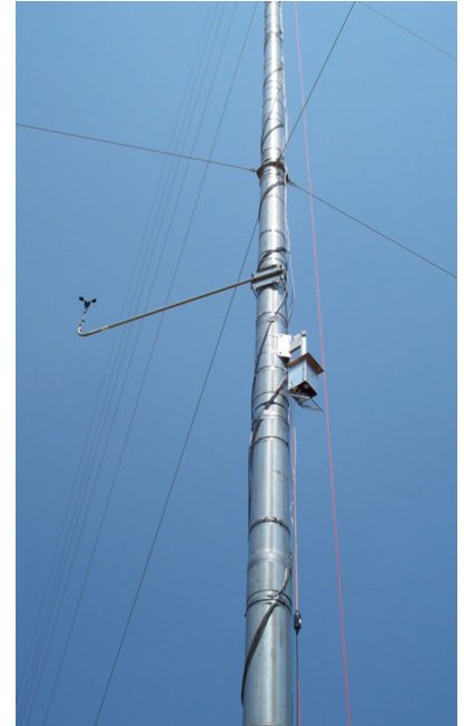
ReBAT upper detector installed on a meteorological tower.
